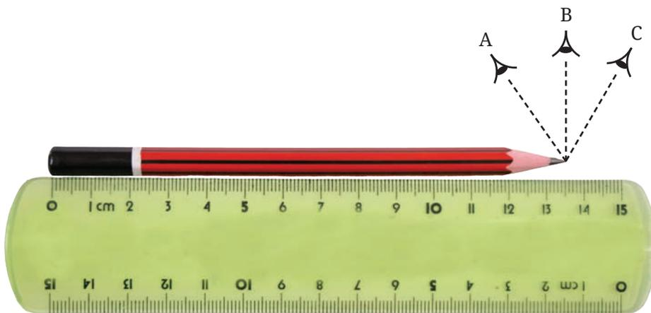
Fig. 5.5: Correct position of the eye is 'B'
