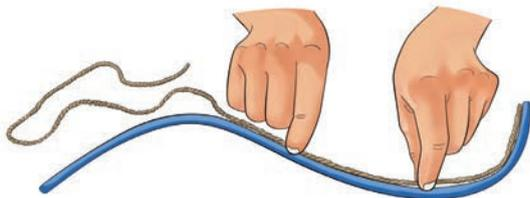
Fig. 5.8: Measuring the length of a curved line
